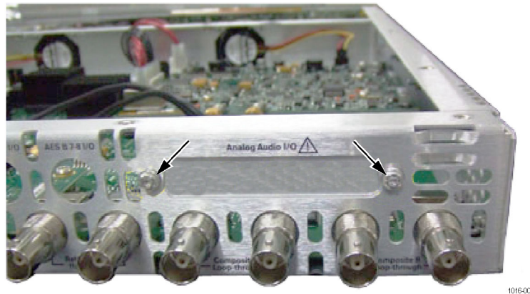
Figure 10: Remove blank cover for audio connector
