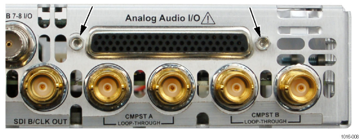
Figure 13: Audio connector retainer posts
